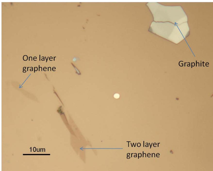
Figure 1: Mechanically exfoliated graphene on SiO<sub>2</sub> imaged with white light using an optical microscope (Photo credit: Nathaniel Safron).
